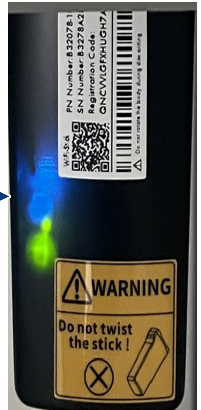
Fig. 50. Connection established – blue LED flashes.
