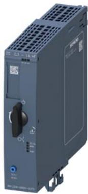
Direct-on-line starter High Feature; Electronic switching; Electronic overload protection up to 0.25 kW / 400 V; Adjustment range 0.3 .. 1 A; PROFenergy; Option: 3DI/LC module
