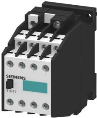
Contactor relay, 80E, DIN EN 50011, 8 NO, screw terminal AC operation 230 V AC 50 Hz, 277 V 60 Hz
