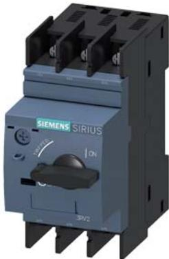
Circuit breaker size S00 for motor protection, CLASS 10 A-release 3.5...5 A
