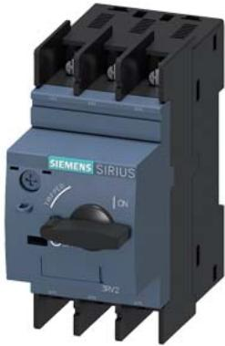
Circuit breaker size S00 for motor protection, CLASS 10 A-release 7...10 A N release 130 A ring cable lug connection Standard switching capacity
