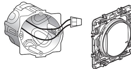
Use a **connector** to connect the two wires.
