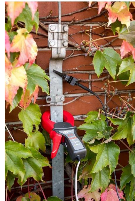
The gap (formed by the faces of the core) should be kept perfectly clean.
