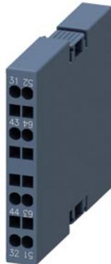
auxiliary switch, lateral, 1 NO + 1 NC, on the left: 51/52, 63/64, on the right: 31/32, 43/44, current path: 1 NC, 1 NO, spring-loaded terminal, for contactors 3RT2 and contactor relays 3RH2
