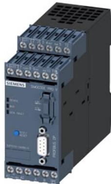
Basic unit SIMOCODE pro V PB PROFIBUS DP interface 12 Mbit/s, RS 485, 4I/3O freely parameterizable, Us: 110...240 V AC/DC, input for thermistor connection Monostable relay outputs, expandable by extension modules
