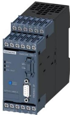
Basic unit SIMOCODE pro V PB PROFIBUS DP interface 12 Mbit/s, RS 485, 4I/3O freely parameterizable, Us: 24 V DC, input for thermistor connection Monostable relay outputs, expandable by extension modules
