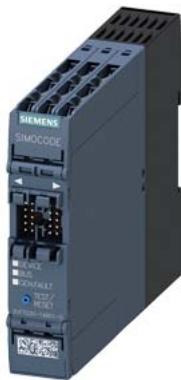
Basic unit SIMOCODE pro S, PROFIBUS DP interface 1.5 Mbit/s, 4I/2O freely parameterizable, Us: 24 V DC, input for thermistor connection Monostable relay outputs, expandable by a multifunctional module
