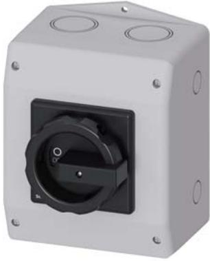
SENTRON, Switch disconnector 3LD, main switch, 6-pole, Iu: 25 A, Operating power / at AC-23 A at 400 V: 9.5 kW, molded-plastic encapsulation for metric screw connection, 1 NC, 1 NO, rotary operating mechanism, black
