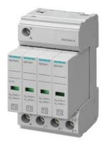
Surge arrester Type 2 Requirement class C, UC 350V Pluggable protective modules 4-pole, 3+1 circuit for TN-S and TT systems Narrow design
