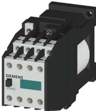
Contactor relay, 44E, DIN EN 50011, for railway applications 4NO+4NC, screw terminal Operating range 0.7...1.25xUS connected to varistor 24 V DC
