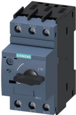
Circuit breaker size S0 for motor protection, CLASS 10 A-release 0.7...1 A N-release 13 A screw terminal Standard switching capacity
