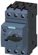
Circuit breaker size S00 for motor protection, CLASS 10 A-release 0.22...0.32 A N-release 4.2 A screw terminal Standard switching capacity
