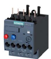
Overload relay 0.28...0.40 A Thermal For motor protection Size S00, Class 10 Contactor mounting Main circuit: Screw Auxiliary circuit: Screw Manual-Automatic-Reset
