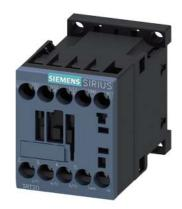
power contactor, AC-3e/AC-3, 7 A, 3 kW / 400 V, 3-pole, 230 V AC, 50/60 Hz, auxiliary contacts: 1 NO, screw terminal, size: S00  $\,$
