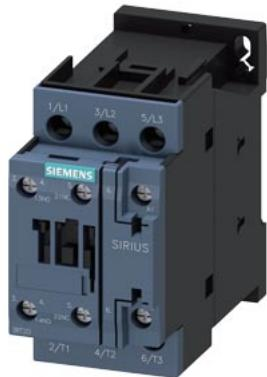
power contactor, AC-3e/AC-3, 25 A, 11 kW / 400 V, 3-pole, 230 V AC, 50/60 Hz, auxiliary contacts: 1 NO + 1 NC, screw terminal
