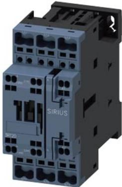
power contactor, AC-3e/AC-3, 25 A, 11 kW / 400 V, 3-pole, 230 V AC, 50 Hz, auxiliary contacts: 1 NO + 1 NC, spring-loaded terminal
