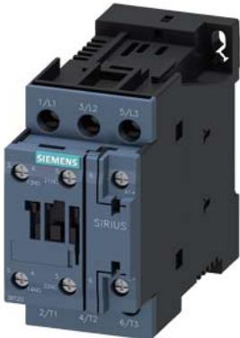
power contactor, AC-3e/AC-3, 17 A, 7.5 kW / 400 V, 3-pole, 200-280 V AC/DC, 50/60 Hz, with integrated varistor, auxiliary contacts: 1 NO + 1 NC, screw terminal, size: S0
