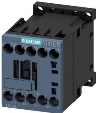
power contactor, AC-3e/AC-3, 12 A, 5.5 kW / 400 V, 3-pole, 110 V AC, 50/60 Hz, auxiliary contacts: 1 NC, screw terminal
