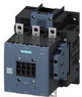
power contactor, AC-3e/AC-3 150 A, 75 kW / 400 V AC (50-60 Hz) / DC Uc: 110-127 V 3-pole, auxiliary contacts 2 NO + 2 NC drive: conventional main circuit: busbar control and auxiliary circuit: screw terminal
