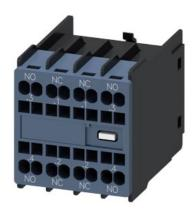
auxiliary switch, on the front, 2 NO + 2 NC, .3/.4, .1/.2, .1/.2, .3/.4, current path: 1 NO, 1 NC, 1 NO, spring-loaded terminal, for contactors 3RT2 and contactor relays 3RH2
