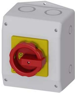
SENTRON, Switch disconnector 3LD, emergency switching-off switch, 3- pole, Iu: 63 A, operating power / at AC-23 A 400 V: 22 kW, Molded plastic encapsulation for metric cable gland, rotary operating mechanism, red/yellow
