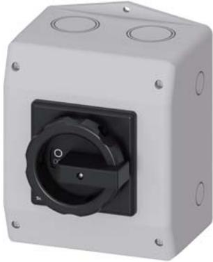
SENTRON, Switch disconnector 3LD, main switch, 3-pole, Iu: 63 A, Operating power / at AC-23 A at 400 V: 22 kW, molded-plastic encapsulation for metric screw connection, 1 NC, 1 NO, rotary operating mechanism, black
