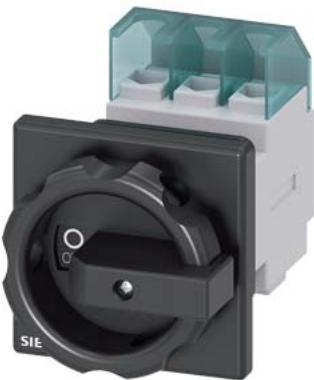
SENTRON, Switch disconnector 3LD, main switch, 3-pole, I<sub>u</sub>: 32 A, Operating power / at AC-23 A at 400 V: 11.5 kW, front-mounted, rotary operating mechanism, black, central mounting 22.5 mm of the handle
