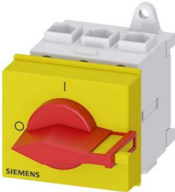
SENTRON, Switch disconnector 3LD, emergency switching-off switch, 3-pole, Iu: 25 A, operating power / at AC-23 A 400 V: 9.5 kW, installation in distribution boards, knob-operated mechanism, Red / yellow, handle direct at the switch
