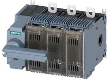
Switch disconnector with fuse 160 A, Size 2, 3-pole for LV HRC fuse Sz. 000 and 00 Front operating mechanism left Complete unit with direct operating mechanism gray flat terminal
