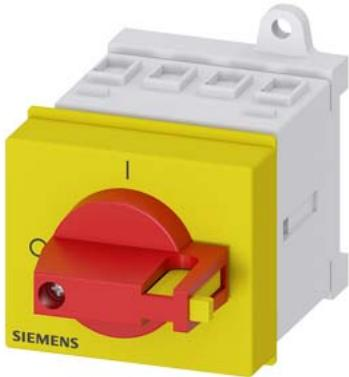
SENTRON, Switch disconnector 3LD, emergency switching-off switch, 3- pole, Iu: 16 A, operating power / at AC-23 A 400 V: 7.5 kW, installation in distribution boards, knob-operated mechanism, Red / yellow, handle direct at the switch
