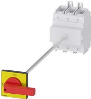
SENTRON, Switch disconnector 3LD, emergency switching-off switch, 3- pole, I<sub>u</sub>=250 A, operating power / at AC-23 A 400 V: 132 kW, floor mounting with door coupling, knob-operated mechanism, red/yellow, 4-hole mounting of the handle
