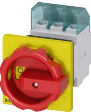
SENTRON, Switch disconnector 3LD, emergency switching-off switch, 3- pole, Iu: 32 A, operating power / at AC-23 A 400 V: 11.5 kW, front-mounted, rotary operating mechanism, Red / yellow, central mounting 22.5 mm of the handle
